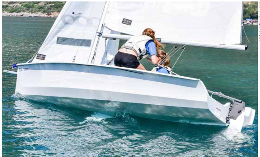
Leeward heel helps with turning towards the wind or can be a nuisance if the boat is kept in a straight line by pulling on the rudder.
