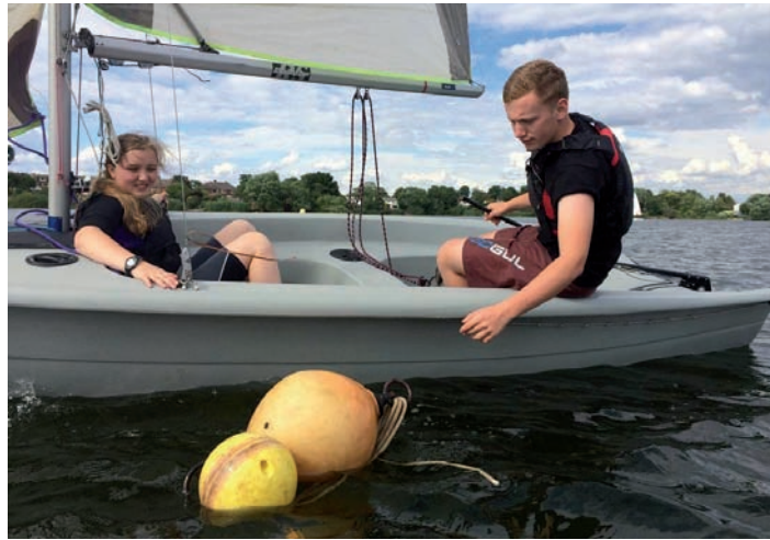
'Spill and fill' to position the MOB by the windward shroud with the boat stopped in the lying-to position.
