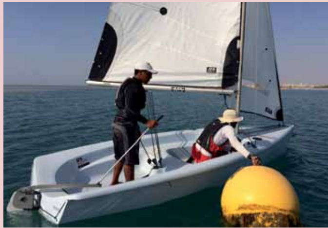
To set sail again, moving the mooring aft can create enough windage on the bow to guide it onto the right course.
